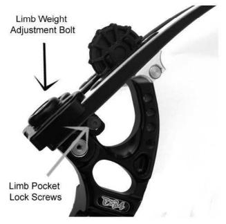
Your bow peak weight can be adjusted approximatly by 7 pounds by turning the limb weight adjustment bolt.
