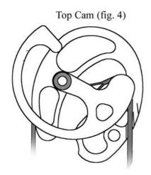
If you find that the cables are not lining up with the timing marks then twisting of the strings and cables are necessary to bring them back into line. This must be done in a suitable bow press. If in any doubt, contact your authorised Merlin dealer.
